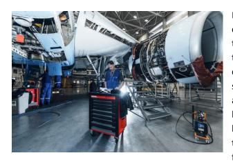
Base maintenance is normally always conducted in a hangar facility and includes all the heavier work and defects not covered on the line maintenance plus the major periodic checks. It is rare for engineers to work in both settings within the same company, but in some airlines it is common for the line to support the base maintenance on nightshifts, and less likely for base maintenance staff to support the line. Aircraft are normally in for anything from a few days to sometimes 6 months
